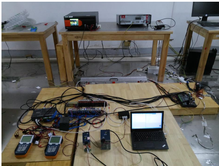
Photograph 11: Electrical Fast Transient/Burst Test Configuration, Signal Port
