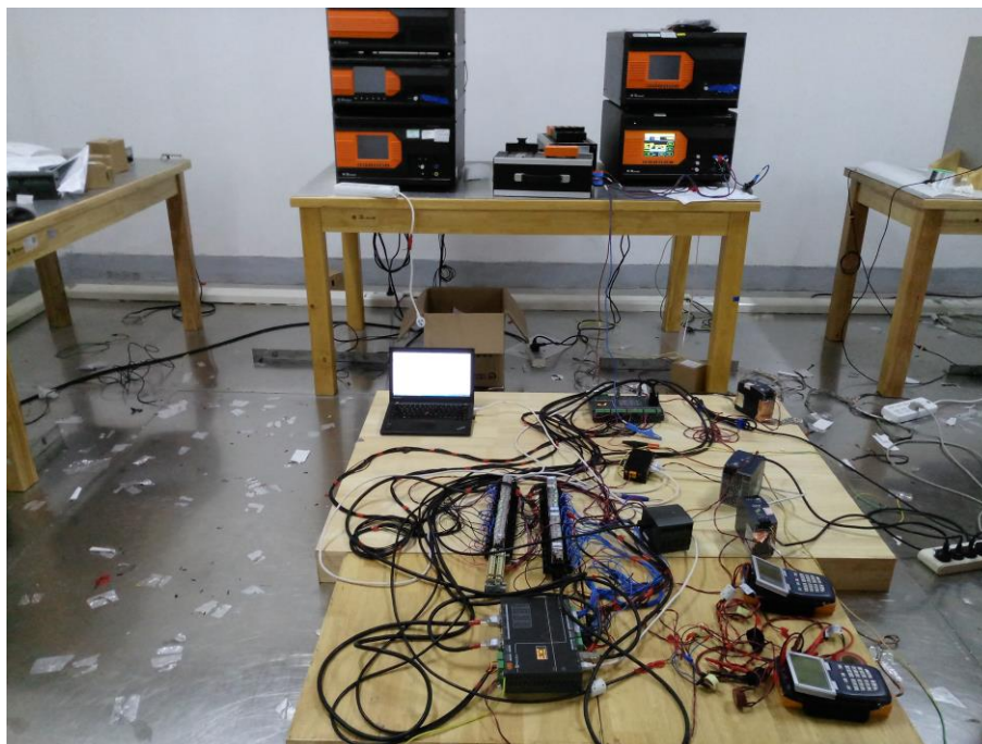
Photograph 14: Voltage Surge Immunity Test Configuration Signal Port
