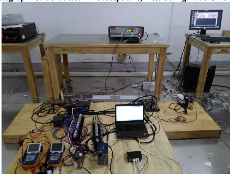
Photograph 15: Conducted RF Susceptibility Test Configuration, AC Line
