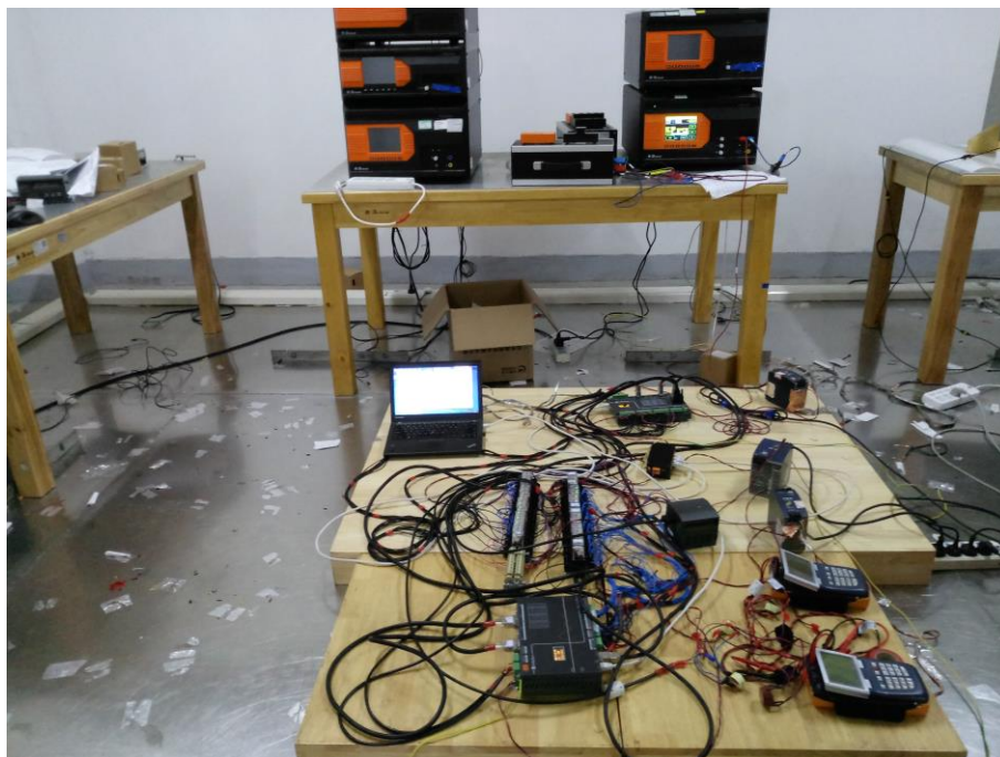
Photograph 13: Voltage Surge Immunity Test Configuration Signal Port
