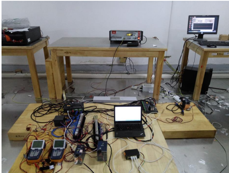
Photograph 17: Conducted RF Susceptibility Test Configuration, Signal Line
