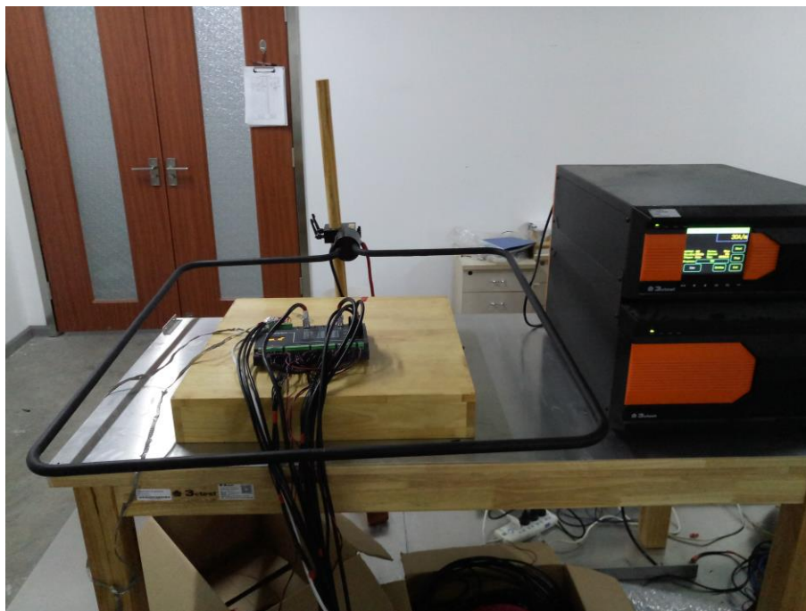
Photograph 22: Magnetic field immunity Test
