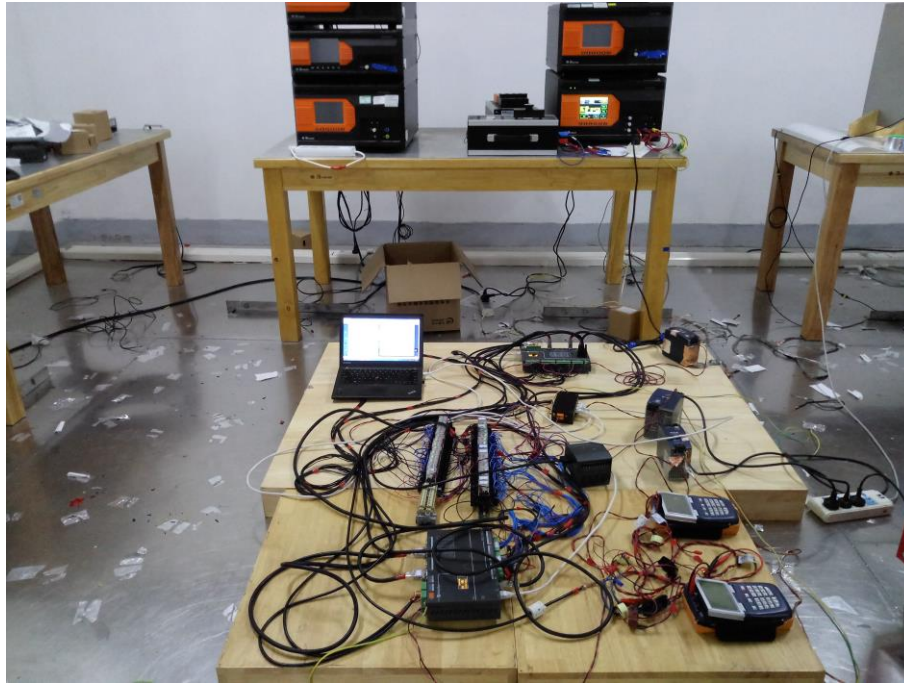
Photograph 12: Voltage Surge Immunity Test Configuration AC Mains Port
