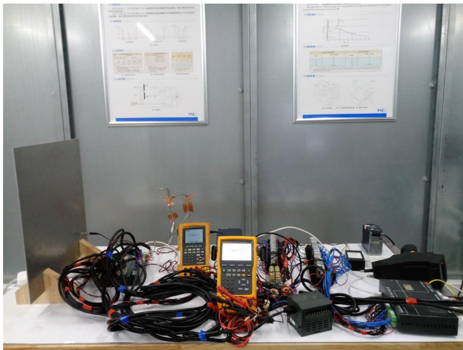
Photograph 6: ESD Test Configuration
