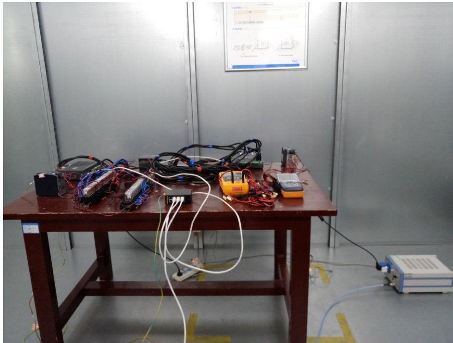
Photograph 2: Conducted Emissions From The AC Mains Power Ports Test Configuration, Front
