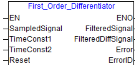
First_Order_Differentiator Functional Block
