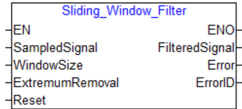
Sliding_Window_Filter Functional Block
