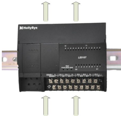
Figure 130 Recommended Heat Dissipation Mode
