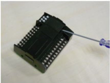
Figure 61 the Removal of Cover
