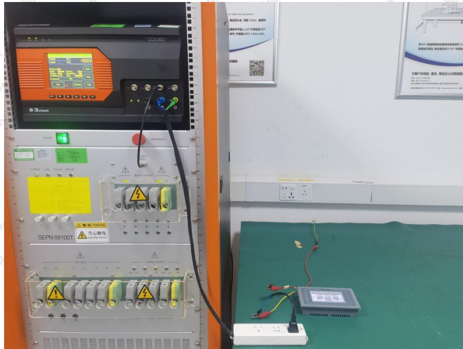
Photo of Surge Immunity Test
