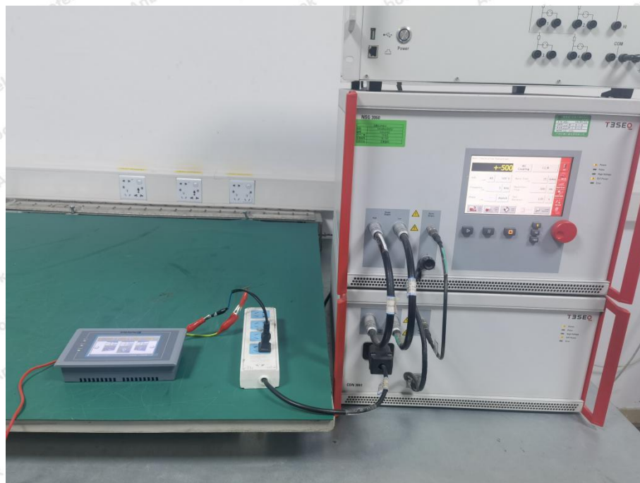
Photo of Electrical Fast Transient/Burst Immunity Test
