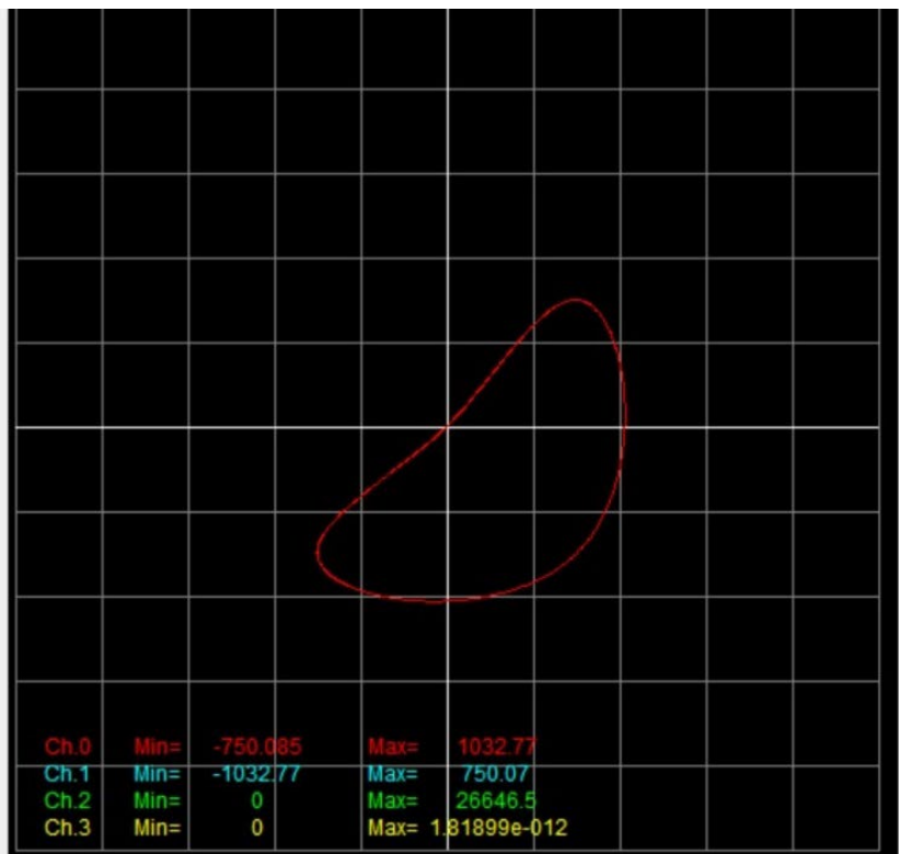
XY-Axis 2D Spline Interpolation Trajectory
