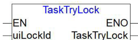
TaskTryLock Functional Block
