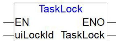
TaskLock Functional Block
